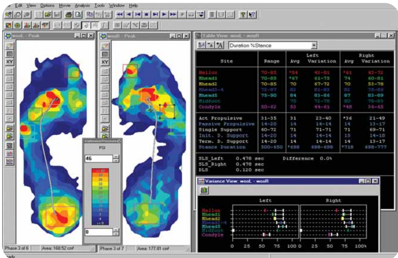
TAM software displays the left and right asymmetries (bottom right), as well as comparing the subject's gait to normal range values at seven sites on the plantar foot (top right).
