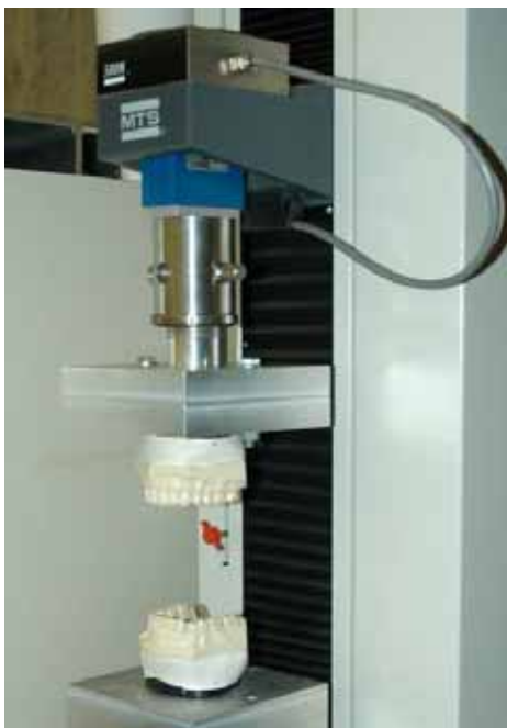
Fig. (1). MTS testing machine - open prior to test.
