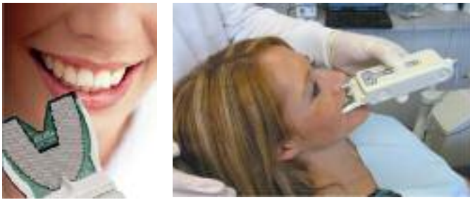
Fig.13. Tekscan sensor with handle and its usage in the operator (Photo courtesy of BioResearch Associates Inc.).
